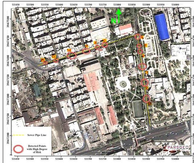
Fig. 6. Detected Anomalies with high degree of risk at both Arab and Pahlavani Streets
